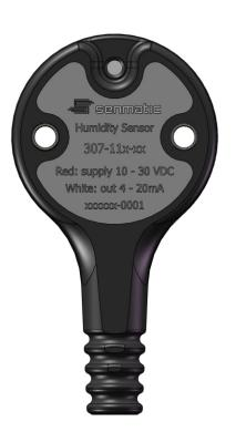
Humidity sensor type MHT is used for measuring of humidity in e.g. refrigeration plants, air-conditioning, ventilating plants and reefer units. Type MHT uses a capacitive element for measuring. A micro controller compensates for unlinearity and the sensor element is tested from factory: In this way accurate measurements are ensured.
