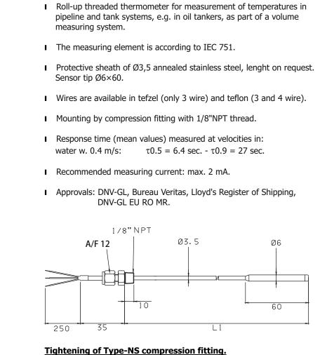
Tightening of Type-NS compression fitting. Tighten the compression part with a torque of 16 Nm.
